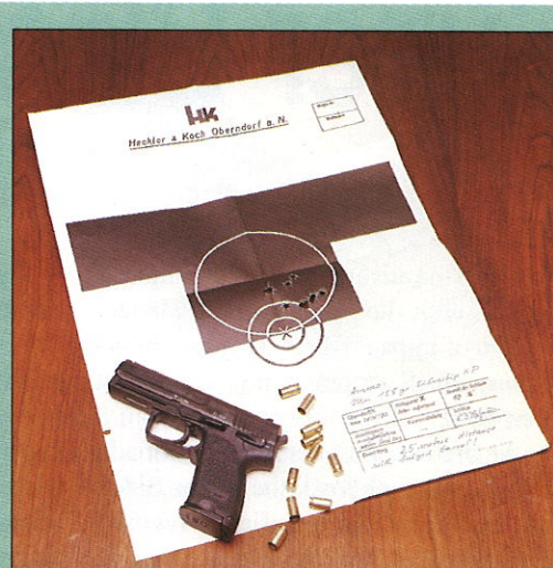
(Above) Target from test firing USP with a bulged barrel. Cutaway (below) shows how the test was conducted. (Bottom) The USP barrel used in the test shows a slight bulge.
