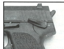
Single control lever. Up for safe, down for fire, all the way down to decock
