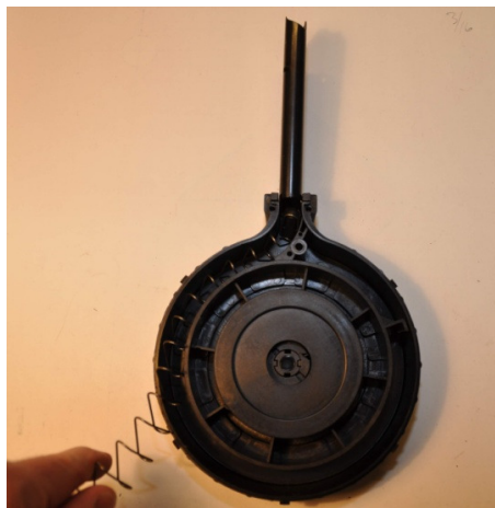
Remove internal follower spring
